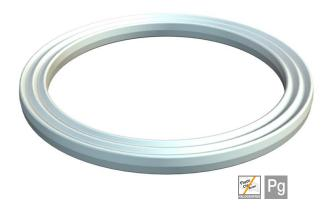
Connection thread sealing ring, in accordance with Part 9 to DIN 46320, however, dimensions may, according to material or function, deviate, suitable for all plastic cable glands with PG connection thread to DIN EN 40430, the internal diameter of the sealing rings are designed so that they can be captively premounted.
