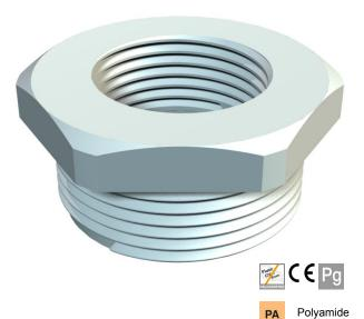
Reduction with PG internal and external thread to DIN 40430 for mounting plastic cable glands on enclosures. Protection class IP54 without additional connecting seal. Protection class up to IP68 possible with additional connecting seal, e.g. Oring or flat sealing ring.
