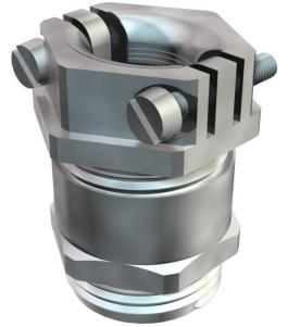
Cable gland with centrically acting transverse clip strain relief in the pressure screw, bend protection of movable cables through strongly rounded pressure screw.
