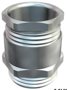
Cable gland with hexagonal intermediate connector, shape C4, to DIN 46320 with Pg connection thread to DIN 40430.
