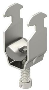
Suitable for all C profile rails with slot width 16–17 mm. Clip, bolt and pressure trough all made of rust-proof stainless steel.
