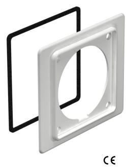
Adapter flange for mounting CEE 16 A sockets. During the mounting of the CEE mounting box, the adapter flange is mounted behind the trunking cover for accessory mounting boxes. Suitable for 400 V CEE 16 A 5-pin 6h, art. no. 6109874.
