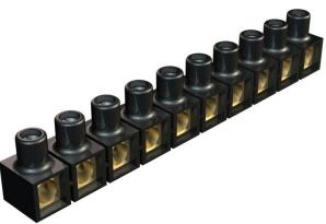
Teminals made of brass, screws of steel, galvanised and transparently passivated, 10-pole, strip separable into individual terminals, open on both sides. Captive upwards screw.
