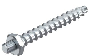
Bolt tie for direct mounting without additional anchors in cracked and uncracked concrete and masonry. M6 connection thread for fastening clips with threaded foot. Construction product tested according to EAD and CE mark, with European Technical Assessment (ETA) and proof of suitability. Load-bearing capacities under fire loads proven up to fire resistance class P120.
