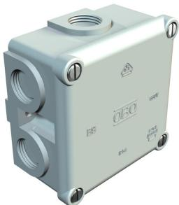
Protection rating IP54, nominal voltage 660 V, nominal cross-section 2.5  $\div$  mm², two fastening holes for screws up to 5 mm Ø on the outside of the box, four cover screws, 7 break-out entries with thread M20 x 1.5, primarily for cable glands with short connecting thread.
