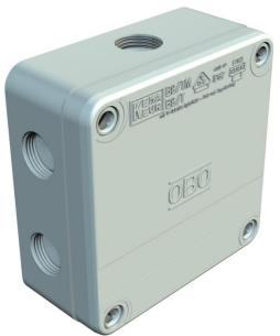
B9/T...: Comprises 2 halogen-free plastics components, 8 threaded entries (PG16) with push-through membrane (for cable diameter up to 15 mm)
