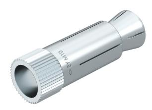
Hollow core anchor "Easy" for mounting in prestressed hollow concrete slabs. When the screw or the nut is tightened, the cone is released from the anchor sleeve and pulled into it. This makes the anchor expand in the hollow space, thereby creating form lock. The hollow core anchor can also be used when the expansion area is not located in the cavity.
