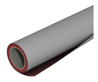
Weatherproof fire protection jacketing made of flexible mesh with fire protection coating to prevent fire spreading via cables and cable support systems. External side grey, internal side red. One roll contains 22 m².
