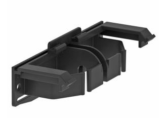
Cover adapter for mounting on trunking bases and fittings of the GAD and Rapid IBIS design device installation trunking series. The cover adapter can be pushed into a guide on the base and is used to accept the trunking cover and keep it at the desired spacing. It is also used for bundled cable exits and can be moved into the lengthwise direction. A maximum spacing of 500 mm between the cover adapters must be maintained.
