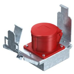
Device support of nominal size 2 with a CEE plug connection 16 A for installation in service outlets and cassettes of nominal size 2, 4, 6 and R7. Device support with protective housing and strain relief. Required minimum installation depth: 190 mm when using a straight connector and 160 mm when an angled connector is used.
