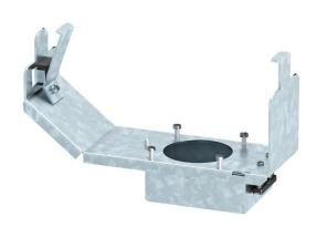
Device support of nominal size 3 for the installation of a CEE plug connection 16 A or 32 A for installation in service outlets and cassettes of nominal size R7, 9 and R9. Device support with protective housing and strain relief. Required minimum installation depth: 190 mm when using a straight connector and 160 mm when an angled connector is used.
