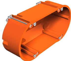
Double device socket, for two service outlets or one double service outlet, with four device screws. Dimensions to DIN 49073-1, for plate thickness 7–35 mm. Standard combination spacing 71 mm, 14 break-out openings for NYM cables, data cables and pipes Ø 20 mm, IP30 protection rating. According to IEC 60670-1, IEC 60670-22 and DIN 49073-1.
