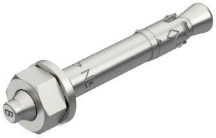
The nail anchor N can be used for multiple fastenings of non-load-bearing systems, indoors and outdoors, in cracked and non-cracked concrete, thereby combining the benefits of a bolt tie with even easier mounting. The nail anchor only needs to be hammered into the drill hole. It is not necessary to apply torque subsequently. When the load occurs, the nail anchor spreads itself and bolts itself in the drill hole.
