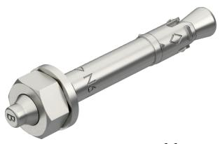
The nail anchor N can be used for multiple fastenings of non-load-bearing systems in areas with highly corrosive impacts in cracked and non-cracked concrete, thereby combining the benefits of a bolt tie with even easier mounting. The nail anchor only needs to be hammered into the drill hole. It is not necessary to apply torque subsequently. When the load occurs, the nail anchor spreads itself and bolts itself in the drill hole.
