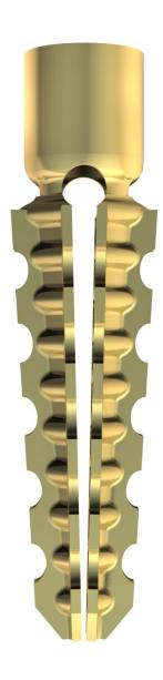
Areas of application: gas concrete, lightweight concrete, Poroton, pumice, plaster, hollow brick and full brick. Can be knocked into porous concrete (gas concrete) of low resistance without drilling. Superbly suited for areas subjected to high temperatures.
