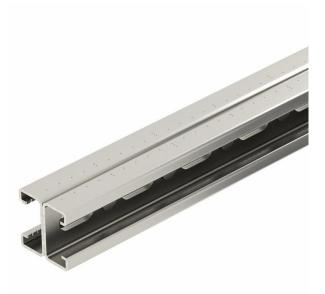
Heavy-duty unistrut with continuous perforation in base, slot width 22 mm. Double version, i.e. two profile rails are interconnected on the base (welded).
