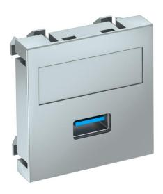
Multimedia support with one USB 3.0 connection socket, straight cable outlet, with labelling panel, USB 3.0 type A socket with screw connection. Support plate with locking fastening, suitable for horizontal and vertical installation in the system environment.
