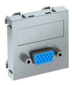
Multimedia support with one VGA connection socket, straight cable outlet, with labelling panel, VGA socket (HD15) with screw connection. Support plate with locking fastening, suitable for horizontal and vertical installation in the system environment.
