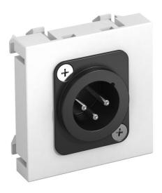
Multimedia support with one XLR connection socket, straight cable outlet, without labelling panel, 3-pin XLR connector with soldered connection. Support plate with locking fastening, suitable for horizontal and vertical installation in the system environment.
