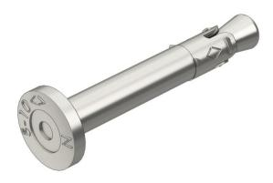
The nail anchor N can be used for multiple fastenings of non-load-bearing systems, indoors and outdoors, in cracked and non-cracked concrete, thereby combining the benefits of a bolt tie with even easier mounting. The nail anchor only needs to be hammered into the drill hole. When the load occurs, the nail anchor spreads itself and bolts itself in the drill hole.
