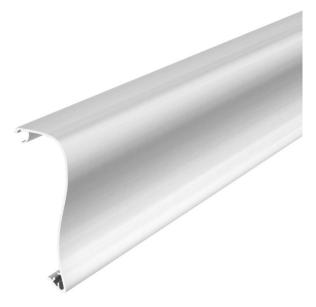
Trunking cover to create a design device installation trunking of the GAD series. "Swing" design version for complete coverage of the system opening and the switching and plug-in devices. The GAD OTA cover adapters are essential and must be planned on the trunking section with a max. spacing of 50 cm. A GAD OTD spacer must be placed between the trunking covers. Standard version in anodised aluminium, different decoration on request.
