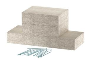
Wall connection collar for PYROLINE® Con D El90 fire protection duct, type PLCD D090810, consisting of fibreglass light concrete, which is resistant to water and frost, for mounting on the fire protection duct in the area of wall and ceiling connections and wall and ceiling penetrations. Consists of 3 single plates (width 100 mm, depth 40 mm). Including countersunk head screws. Including counter-sunk head screws.
