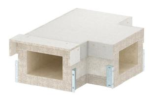
T piece for PYROLINE® Con S El90 fire protection duct, type PLCS D091220, consisting of fibreglass light concrete which is resistant to water and frost, for the creation of T branches in the duct route. Mounted connectors ensure quick mounting in situ, whilst loosely placed covers ensure quick inspection and reassignment.
