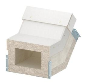
Vertical bend, rising, for PYROLINE® Con S El90 fire protection duct, type PLCS D091220, consisting of fibreglass light concrete which is resistant to water and frost for the creation of vertical changes of direction (45°) of the duct. Mounted connectors ensure quick mounting in situ, whilst loosely placed covers ensure quick inspection and reassignment.
