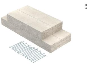
Wall connection collar for PYROLINE® Con S El90 fire protection duct, type PLCS D090810, consisting of fibreglass light concrete, which is resistant to water and frost, for mounting on the fire protection duct in the area of wall connections and wall penetrations. Consists of 4 single plates (width 50 mm, depth 30 mm).
