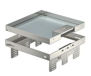
Height-adjustable cassette, decoupled from the floor, of nominal size 9, with cord outlet, for the installation of accessories in dry-cleaned floors indoors, for mounting in underfloor boxes UZD250-3 or UZD350-3, either in conjunction with a mounting cover DUG../9 or in UGD250-3/9 or UGD350-3/9. Mounting takes place using height-adjustment brackets (order separately) in the aluminium frame profile of the underfloor boxes.
