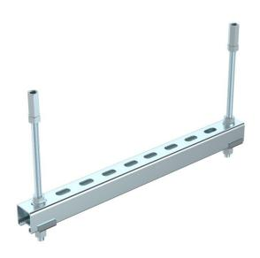
Suspension and fastening material, made of steel, to create the first support of pass-through installations in fire insulation. Mounting of the pendulum with threaded rods under the ceiling. A maximum of two layers can be mounted with connection sleeves from two sets. The support constructions must be arranged on both sides of the wall at the prescribed distance to the insulation system. Including 2x MMS-plus I 7.5 x 40
