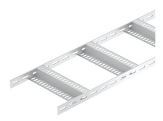
Shipbuilding cable ladder with perforated side rail of side height 40 mm with welded, perforated Z rungs.
