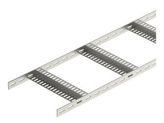
Light-duty shipbuilding cable ladder with perforated side rail of side height 35 mm with welded, perforated Z rungs. Load tested according to IEC in conjunction with connector, type SLV. Bends on request.
