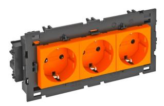
Protective contact socket with connection to side, triple  $0^{\circ}$ , with increased touch protection, with screwless terminals, 2-pin, 16 A, 250 V~, with connection terminals to IEC 60884-1, suitable for the installation in Rapid 80 device installation trunking systems.
