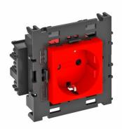
Protective contact socket with connection to side, Single 0°, with increased touch protection, with screwless terminals, 2-pin, 16 A, 250 V $\sim$ , with connection terminals to IEC 60884-1, suitable for the installation in Rapid 80 device installation trunking system.
