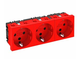
Protective contact socket, triple  $0^\circ$ , encoded version, with increased touch protection, with screwless terminals, 2-pin, 16 A, 250 V~, with connection terminals according to IEC 60884-1.
