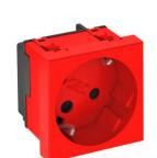
Protective contact socket Single 33°, encoded version, with increased touch protection, with screwless terminals, 2-pin, 16 A, 250 V~, with connection terminals according to IEC 60884-1.
