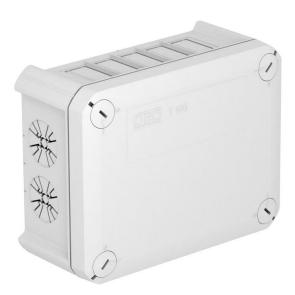
Junction box for 6 Wieland sockets, 3-pin, for the connection of cables indoors and in protected outdoor areas. Rectangular design with knock-out entries to the sides and knock-out entries in the bottom. Suitable for wall and ceiling mounting and on mounting panels. With the option of fastening inside and to mount via the corner domes. Cover with quick lock, sealable. Made from halogen-free and UVresistant materials.
