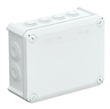
Junction box for the connection of cables and lines indoors and in protected outdoor areas. Rectangular design with plug-in seals to the sides and knock-out entries in the bottom. Suitable for wall and ceiling mounting and on mounting panels. With the option to fasten inside and to mount via the corner domes. Cover with quick lock, sealable. Flame-resistant type made from special polypropylene.
