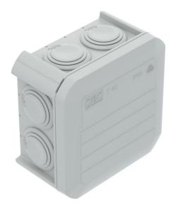
Junction box for the connection of cables and lines indoors and in protected outdoor areas. Square design with plug-in seals to the sides and knock-out entries in the bottom. Suitable for wall and ceiling mounting and on mounting panels. With the option to fasten inside. With fixed clamping cover. Flame-resistant type made from special polypropylene.
