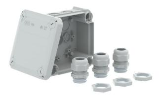
Junction box for the connection of cables and lines indoors and in protected outdoor areas. Square design with knock-out entries to the sides and knock-out entries in the bottom. Suitable for wall and ceiling mounting and on mounting panels. With the option to fasten inside and to mount via the corner domes. Cover with quick lock, sealable. Made from halogen-free and UV-resistant materials.
