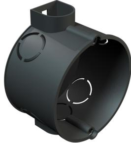
Device socket with torsion-resistant guaranteed standard combination spacing of 71 mm (to DIN 49 073-1) through Snap-lock coupling. 7 break-out openings for cables and pipes Ø 20 mm and Ø 25 mm. Combinable for spreading and screw fastening, low-lying plaster brackets, device bolt spacing 60 mm, for screw fastening with 3.2 mm self-tapping screws, with 2 screw bosses without screws, protection rating IP20.
