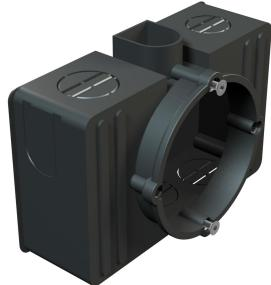
Device/connection socket with increased socket volume on both sides of the device installation opening to accept connection terminals. Torsion-resistant guaranteed standard combination spacing of 71 mm (to DIN 49 073-1) through snap-lock coupling. Break-out openings for cables and pipes of up to Ø 21 mm, low-lying plaster brackets, device bolt spacing 60 mm, for screw fastening with 3.2 mm self-tapping screws, with 4 screw bosses and 2 device screws, protection rating IP20.
