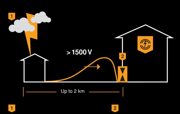
A local lightning strike creates additional high magnetic fields, which in turn induce high voltage peaks in cable systems. Damage can be caused within a radius of up to 2 km around the lightning impact point.
