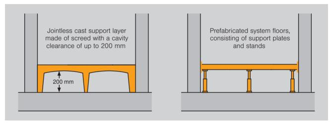
Definition of system floors: Cavity floor (left), raised floor (right)
