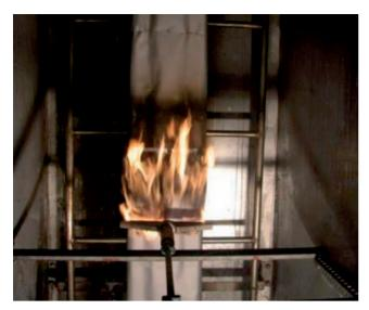
Testing of the cable bandage
