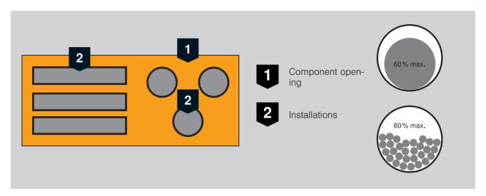
A maximum of 60% of the area may be assigned with cables, support systems, pipes, etc.
