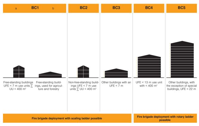
UFE: Upper floor edge of the highest storey UU: Use units, BC: Building classes
