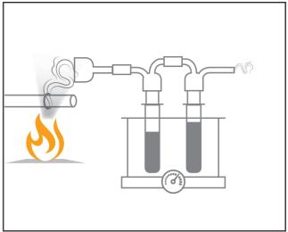
Measurement of the pH value when burning the insulating material
