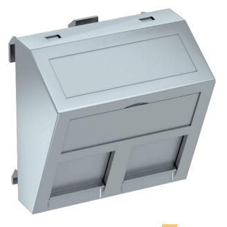
Data technology support with slanting outlet and locking slider to accept two data technology connection modules with RJ45 socket. The locking fastening is suitable for horizontal and vertical installation in the system environment. Type A has a mounting opening of  $20.10 \times 14.80 \, \text{mm}$  and is designed for direct fastening of the data connection modules in the mounting opening.
