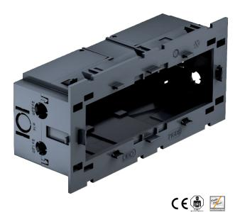
Front locking triple accessory mounting box for Modul 45® system, with folding, and also removable, base for time-saving cable connection, with feed openings for cable diameters of up to 14 mm.
