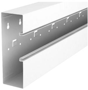
GS device installation trunking for mounting on the wall or on fastening panels. The GS device installation trunking possesses self-contacting locking straps to accept a sheet steel partition. The equipotential bonding between the trunking bases takes place using the trunking coupler. The protective measure and the equipotential bonding is guaranteed between the cover and the base by the self-contacting trunking cover. The real system opening is 76.5 mm.
