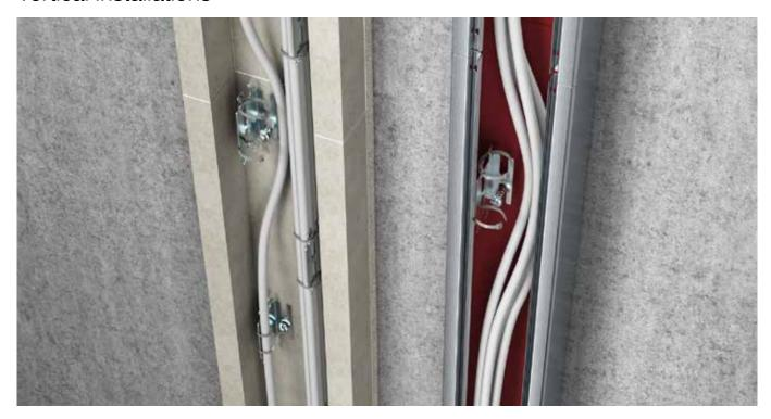
Universal cable bracket for the vertical installation of cables in PYROLINE® Con fire protection ducts made of fibre glass-reinforced, lightweight concrete, as well as PYROLINE® Rapid made of sheet steel with an internal coating.
