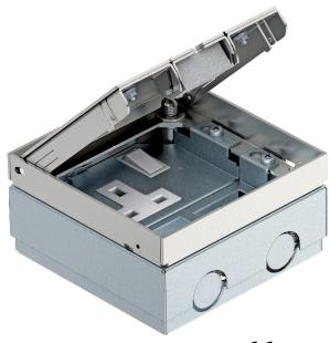
Square installation unit for use in dry-care cavity and screed floors in indoor areas. Installation housing with pre-marked insertion openings for pipes (M25). Cover adjustable to top edge of floor covering using four height-adjustment supports. The minimum installation depth is 75 mm, the height-adjustment range +20 mm.
